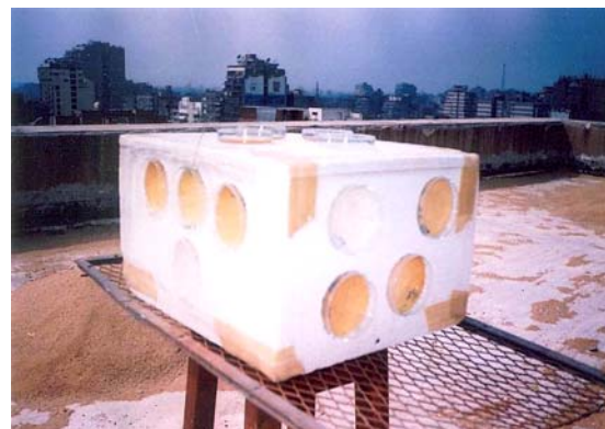
Fig. 1 A polystyrene cube with Petri dishes containing the different fungal media
